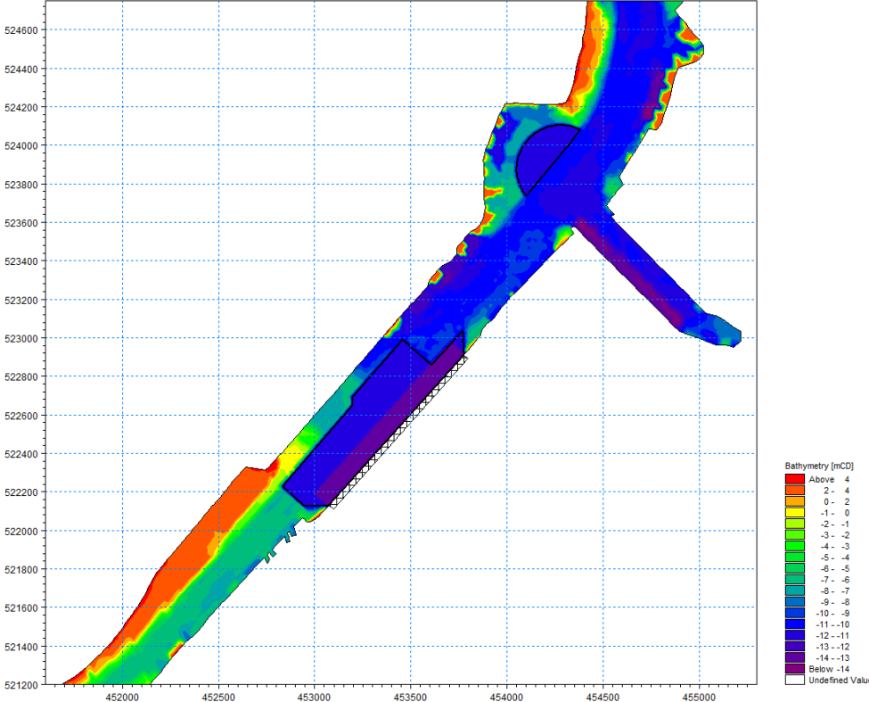
Figure 4.2: Model Scheme Bathymetry
